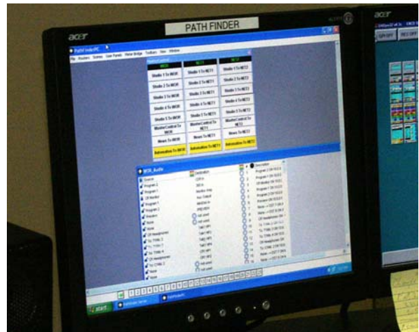
The computer screen for Axia's Pathfinder, WOR's studio switcher and all around system information shuttling device.
